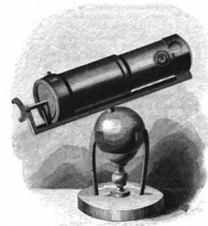
Newton's reflector, the first reflecting telescope
