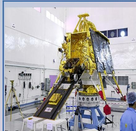
Figure 1: Rover Pragyan mounted on the ramp of Vikram lander
